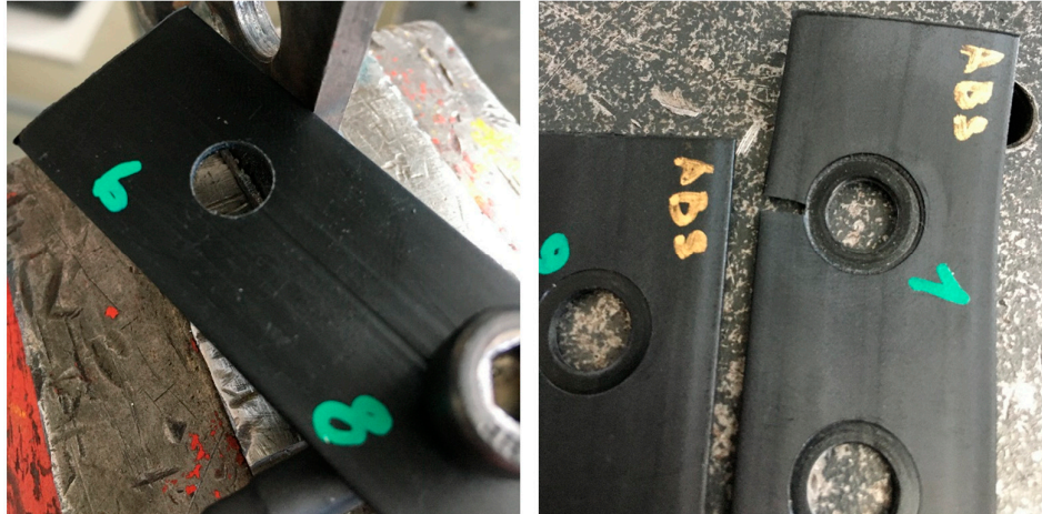
Figure 8. Detail of the sample before the test and damage to the sample during the test (right).
