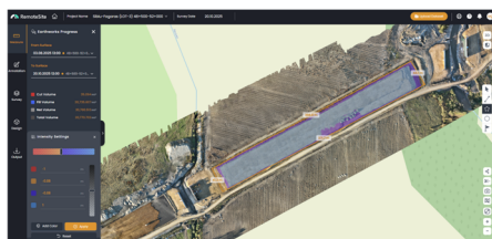
Figure 6. Orthomosaic Map Generated from Drone-Based Photogrammetry.
