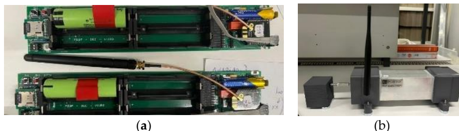
Figure 12. Displacement sensor: (a) interior board with batteries; (b) sensor casing.
