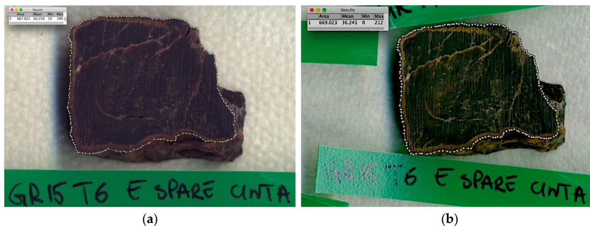
Figure 2. An example of how the surface area changes were calculated using the ImageJ software: (a) the initial area of sample T6 E; (b) the same area after conditioning in the climate at 85% RH.
