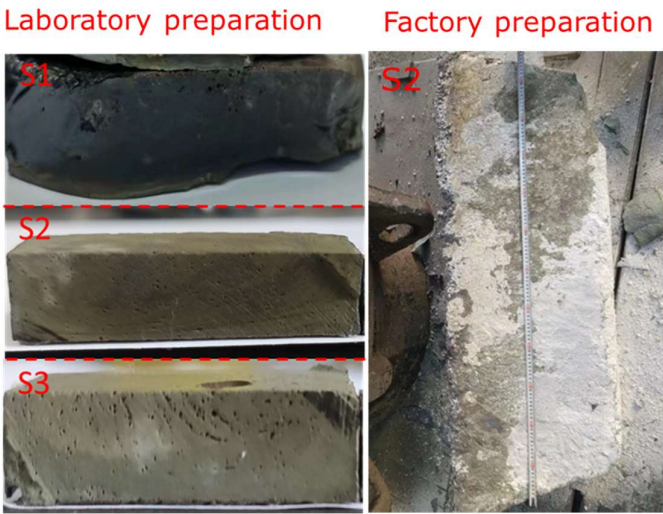
Figure 4. Photos of laboratory and factory prepared (middle position size: 1150 × 350 × 500 mm) cast stone samples.
