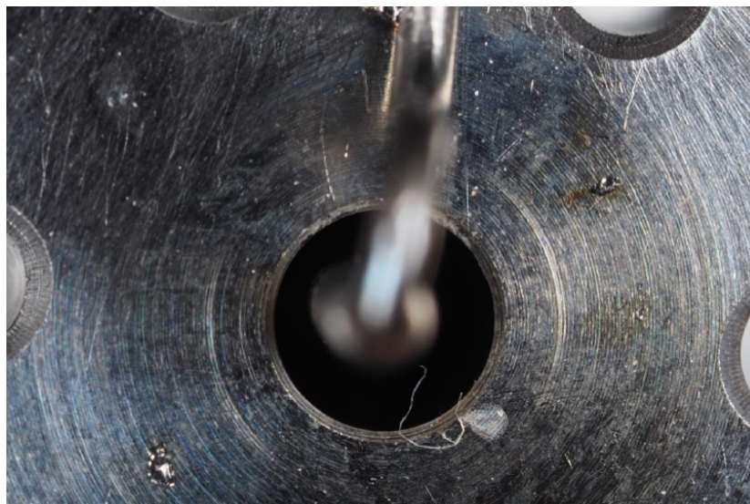
Figure 8. Photo of the RF pickup installed in the accelerating structures.
