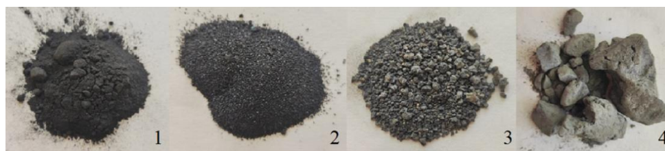
Figure 2. Metallurgical slags: 1) slag storage 1 of the former lead plant, 2) slag storage 2 of the former lead plant, 3) slag storage 3 of the former lead plant, 4) slag storage of the Zhezkent MPP.
