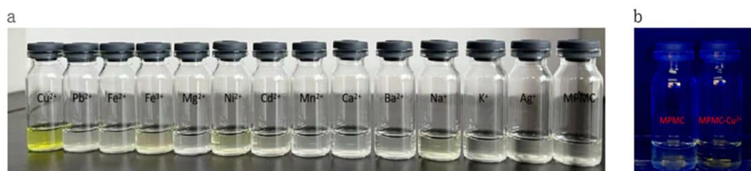
Figure 2. (a) Colorimetric performance of sensor MPMC (1 mM) upon addition of different metal ions (including \text{Cu}^{2+} , \text{Pb}^{2+} , \text{Fe}^{3+} , \text{Fe}^{2+} , \text{Mg}^{2+} , \text{Ni}^{2+} , \text{Cd}^{2+} , \text{Mn}^{2+} , \text{Ca}^{2+} , \text{Ba}^{2+} , \text{Na}^{+} , \text{K}^{+} , \text{Ag}^{+} ) (1 mM) in EtOH/ \text{H}_2\text{O} ( v/v = 1/1 ) solution; (b) color change induced upon addition of \text{Cu}^{2+} under 365 nm UV lamp.
