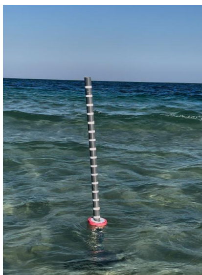
Figure 3. Calibrated rod and small buoy used for on-site wave motion and height measurements.
