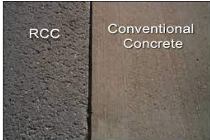
Figure 6. Fly ash RCC rough surface, as compared to conventional concrete [72]
