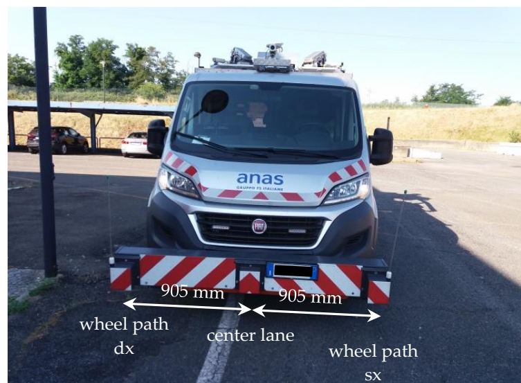
Figure 6. “Cartesio” front view; the profilers are mounted on a bar in front of the vehicle
