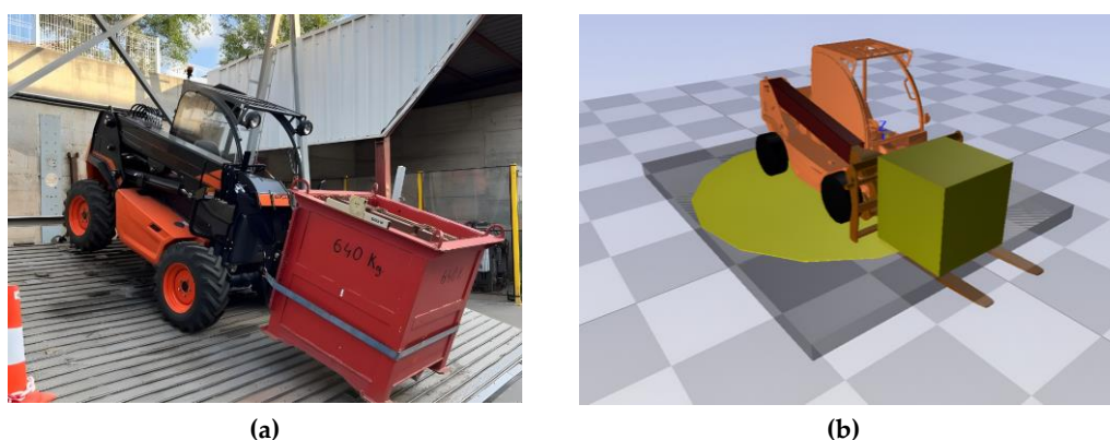
Figure 1. (a) Telescopic machine on Tilting Platform, Source: AUSA (b) Virtual BG-3D Model. (20-Sim animation tool) of Telescopic machine on tilting virtual Platform in a horizontal position.
