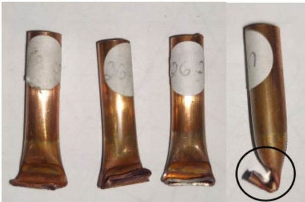
Figure 18. Tubes T4P4 bent after leak testing.
