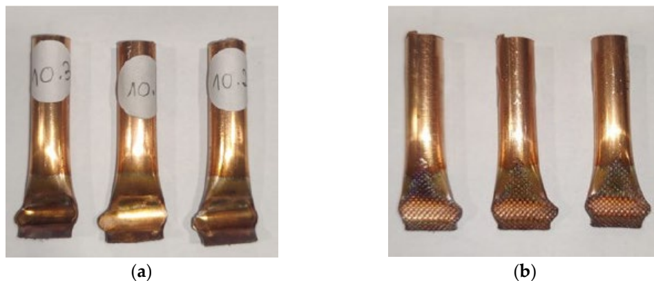
Figure 15. (a) T3P4.5 tubes after welding (sonotrode side); (b) T3P4.5 tubes after welding (anvil side).
