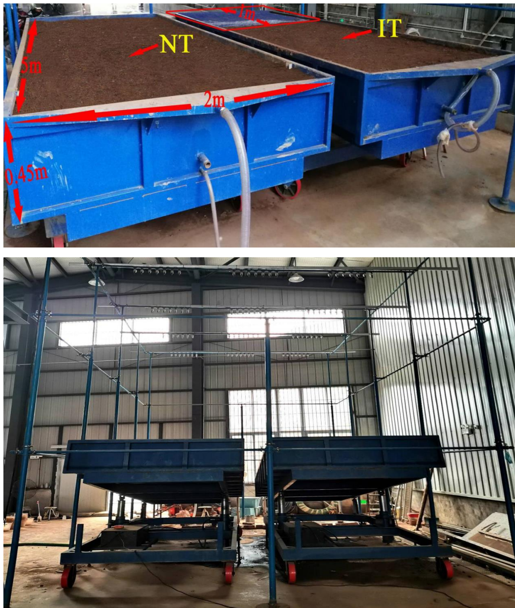
Figure 1. Different tillage intensity treatments (a) and Rainfall simulation (b).
