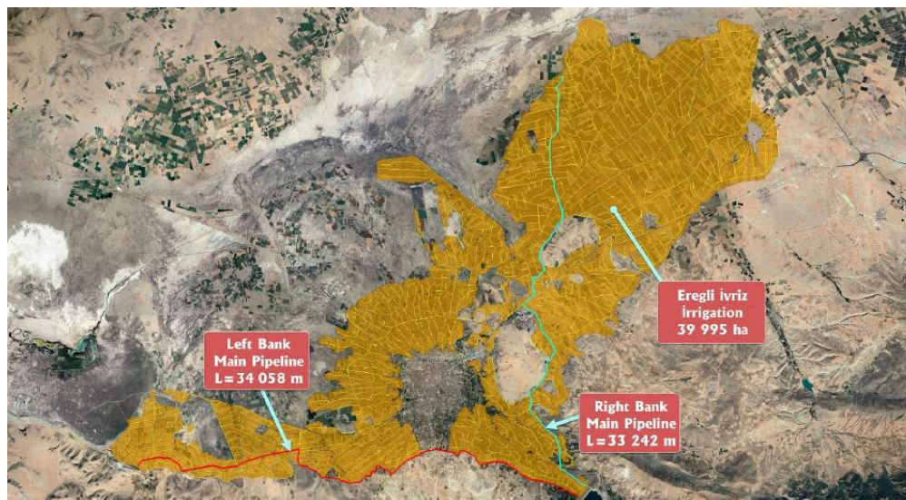
Figure 1. The Ivriz irrigation scheme in Türkiye, highlighting the project’s command area and key pipeline infrastructure.
