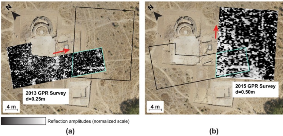
Figure 4. (a) Location and results of 2013 survey (profile spacing of 0.25 m). (b) Location and results of 2015 survey (profile spacing of 0.50 m). The base map is an orthophoto of Horta da Torre remains taken in 2016. The excavations took place after the GPR surveys. Arrows indicate the direction of the profiles. All the results show reflection alignments suggesting the existence of wall-type structures. The difference in profile spacing is visible in the two datasets; it mainly affects spatial resolution.
