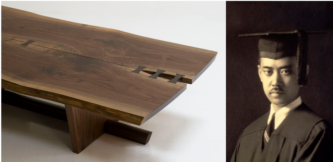
Figure 14. George Nakashima’s Butterfly-Fitting Table Joint (Sakura Seisakusho).
