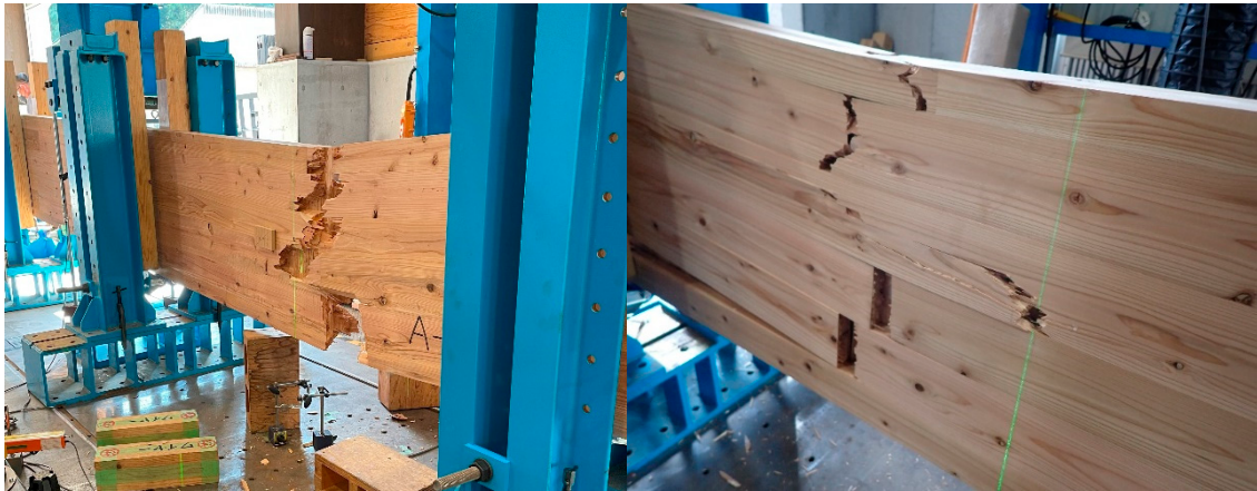
Figure 27. Failure Modes of Pressed (left) and Unpressed (right) Specimens (Authors).
