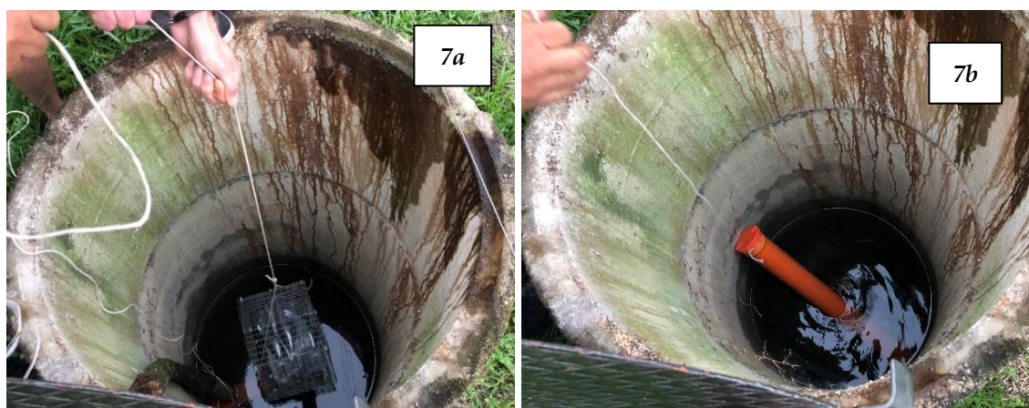
Figures 7a and 7b: Positioning of the cage and one of the PVC pipes inside the well in the vineyard, with the samples immersed at a depth of approximately 3 m.
