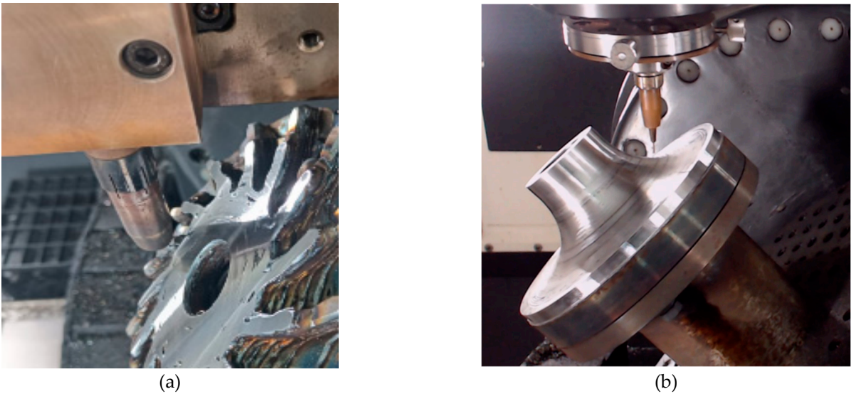
Figure 7. (a) MIG torch while planar 5-axis deposition; (b) Laser with conformal 5-axis deposition.
