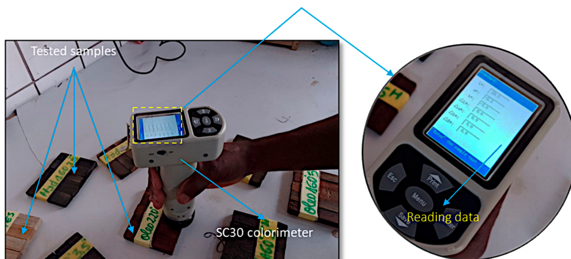
Figure 2. Experimental setup for CIELab color measurements on treated and untreated Dabema.
