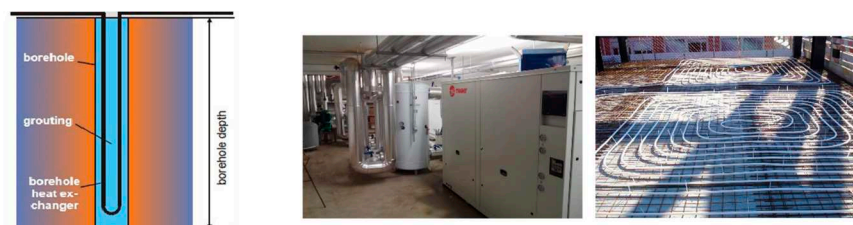
Figure 1. Illustration of GSHP system components: Primary circuit (on the left) (adapted from Socaciu, 2012), Heat pump (in the middle) and secondary circuit (on the right).
