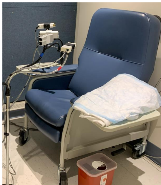
Figure 3. Photograph of the testing environment with the various generations of the Senseair devices oriented in several locations in front of the participant's face.
