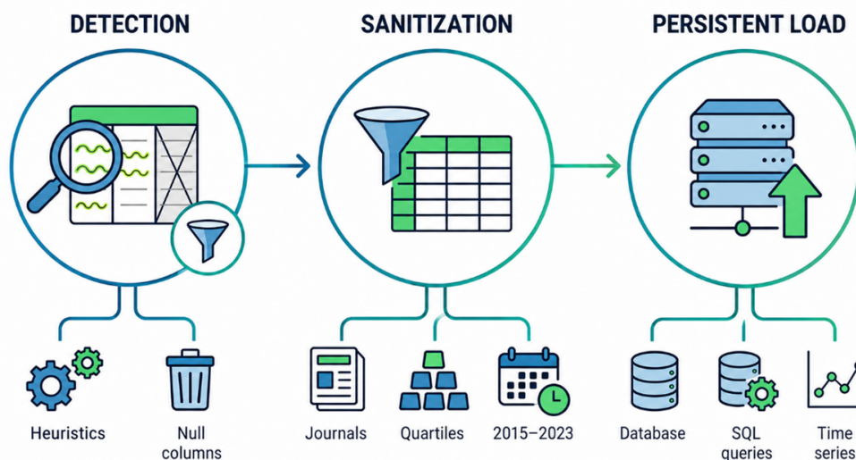
Figure 3. Deterministic Ingestion Pipeline. The three stages Detection, Sanitization, and Persistent Load transform raw heterogeneous sources (via heuristics and null-column removal) into a clean, schema-compliant dataset stored in the database and ready for SQL queries and time-series analysis.
