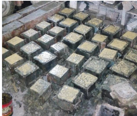
Figure 4: Concrete cubes in molds after casting and before demolding.
