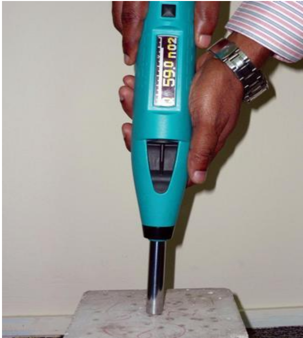
Figure 6: UPV (left) and Rebound Hammer Tests on Cubes (right)
