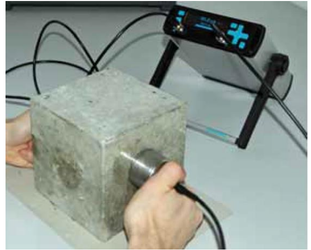
Figure 6: UPV (left) and Rebound Hammer Tests on Cubes (right)
