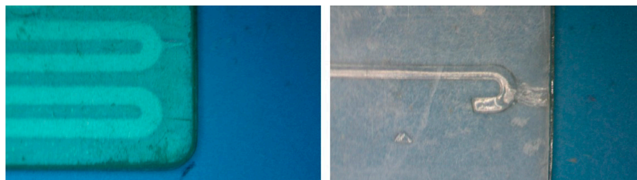
Figure 6. Layer separation and leakages in the microfluidic structure when pressure was applied to remove the uncured resin from the microchannels.
