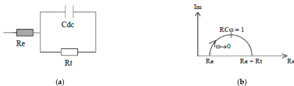
Figure 7. a. Equivalent circuit used in the calculation of the R_e , R_t and C_{dc} parameters. b. Determination of different parameters on the Nyquist diagram.
