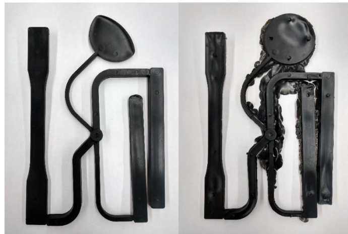
Figure 2. Examples of defects short shot, flash, and sink marks.
