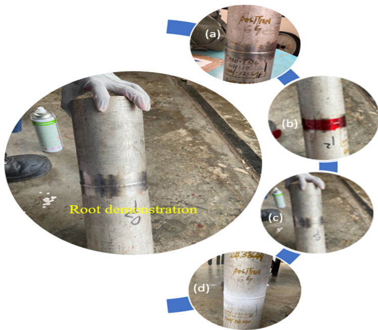
Figure 7. (a) Surface pre-cleaning; (b) Penetrant drawn into flaws by capillary action; (c) Dwell time and removal of excess penetrant; (d) Developer application reveals flaws through visible indications.
