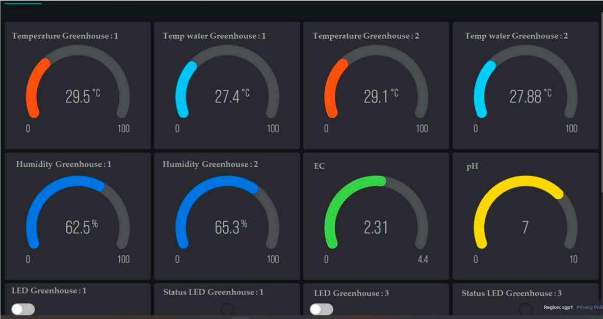
Figure 4. A dashboard is employed for the display of data and management of system operations via the Blynk IoT platform.
