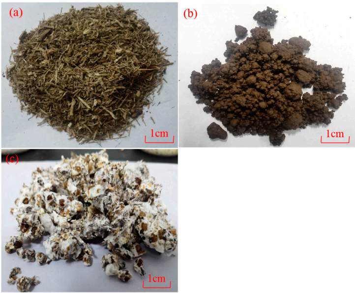
Figure 1. Pictures of substrate filler materials: (a) bagasse, (b) SS, (c) ready-made mycelium.
