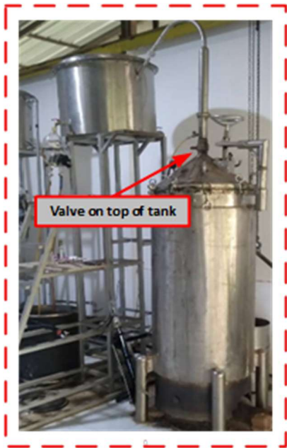
Figure 4. Position of the distillation vessel top valve during RWASD operation.
