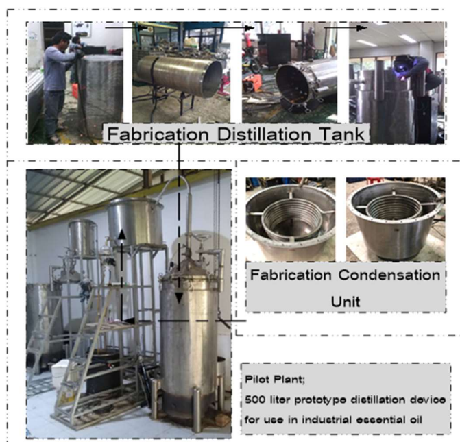
Figure 11. Schematic diagram of the 500-liter essential oil distillation unit assembly and construction.
