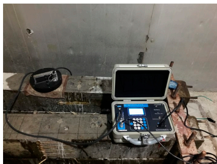
Figure 5. Photo of the corrosion measurement system for the steel bars.
