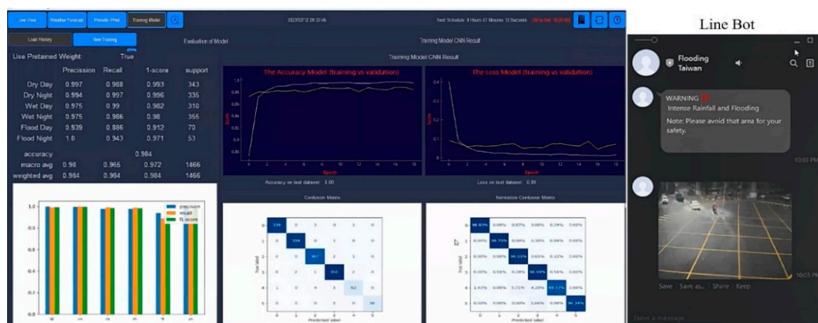
Figure 14. An example of a web interactive flood classification application with automatic Line message generation based on predicted results.
