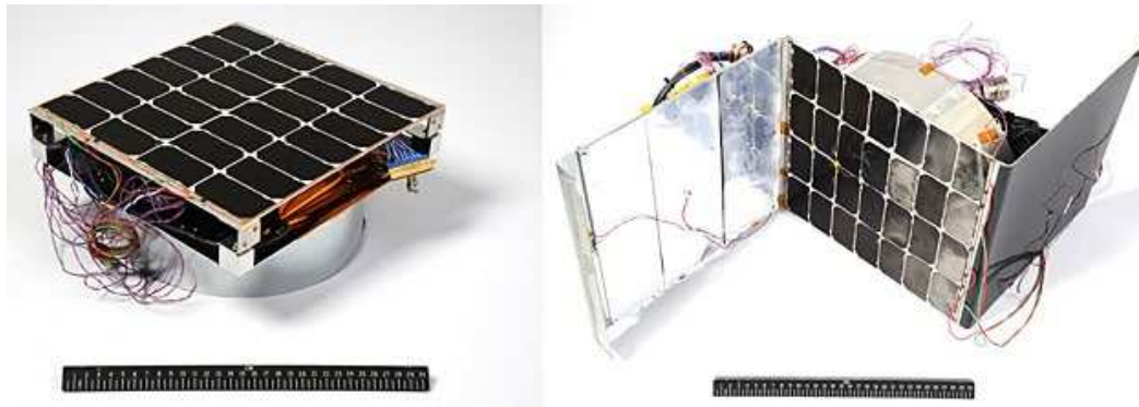
Figure 2. Space based solar sandwich module (left); sandwich step module equipped with more robust thermal radiators. Reprinted from [6,7].
