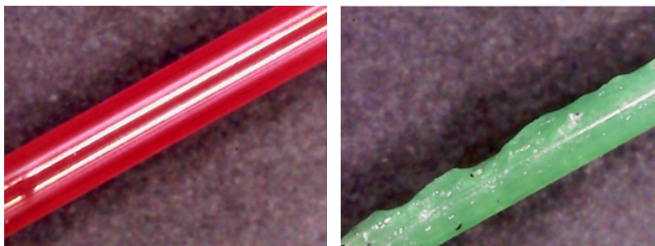
Figure 6. Optical fibers: left figure in good condition and right figure with microbending and dirt.
