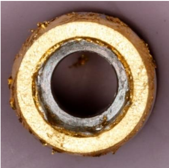
Figure 1. Milled cobalt chrome with gold on the fitting surface.
