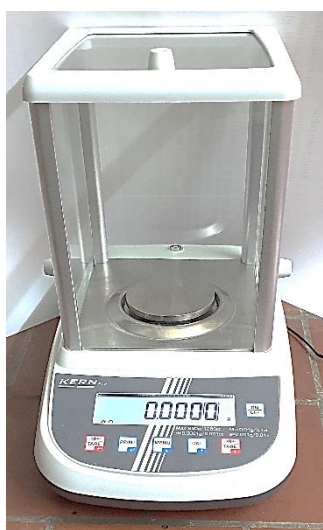
Figure 10. Kern ABS 220-4N analytical balance.
