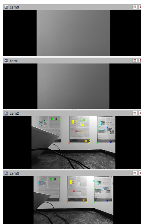
Figure 6. The multi-camera setup during robustness testing: cam0 and cam1 (Stereo 1); cam2 and cam3 (Stereo 2).
