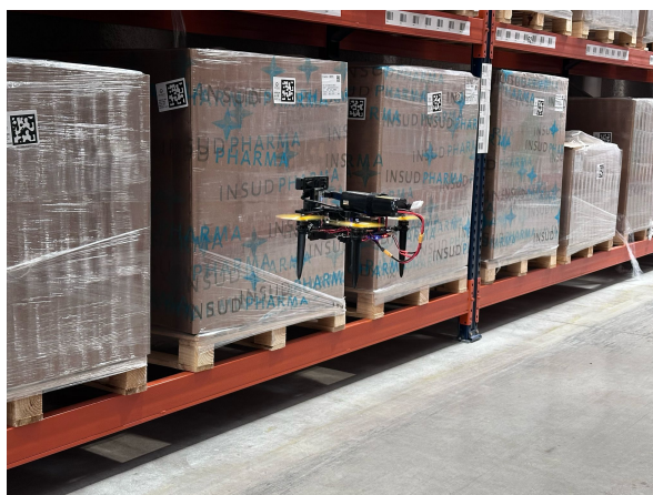
Figure 7. Dronomy's quadcopter flying with our VIO implementation while performing an inventory in a warehouse.
