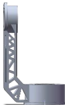
(c) Smoothed topology-optimized structure configuration for compliance minimization considering volume fraction constraints
