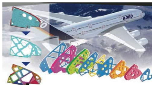
Figure 2. Optimization design of the topology, shape, and dimensions of the A380 wing ribs.
