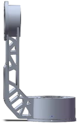
(a) Smoothed topology-optimized structure configuration for volume minimization considering displacement constraints
