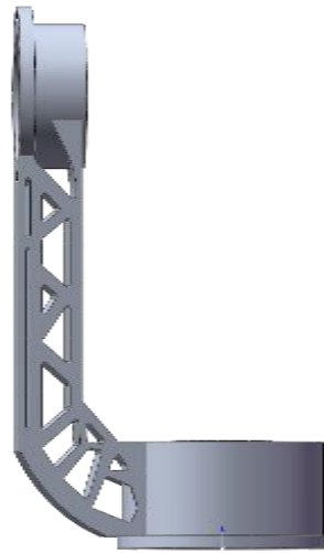
(a) Smoothed topology-optimized structure configuration for volume minimization considering displacement constraints
