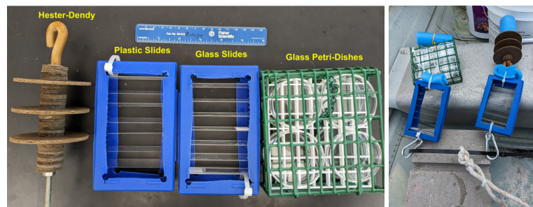
Figure 2. Construction of the sampling apparatus and substrate deployments used to collect polyp colonies of Craspedacusta sowerbii . (a, left) The substrates utilized in the apparatus, including a Hester-Dendy apparatus with three evenly spaced masonite discs, separated by smaller masonite discs, microscope slide boxes with the sides cut out used to hold glass and plastic slides, and a metal cage holding eight petri dishes, with four visible. (b, right) The entire setup with all substrates attached to a zip tie looped through a cinder block.
