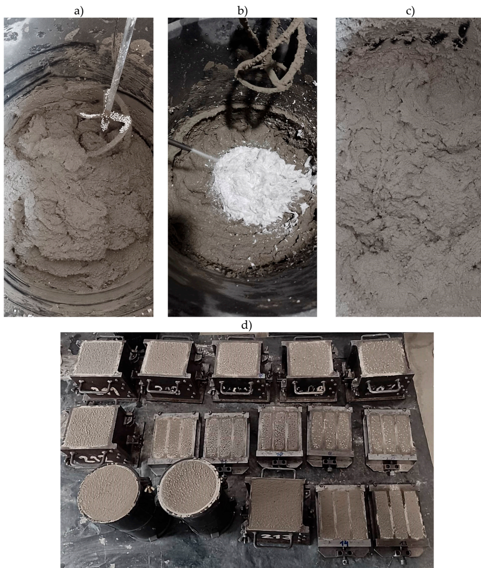
Figure 2. Samples production process a) mix of light plaster mortar with polystyrene granulate addition, b) adding foam to light plaster mortar with polystyrene granulate addition, c) foamed mortar mix, d) samples with foamed mortar in steel moulds (own photos).
