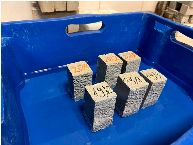
Figure 5. Sorptivity test of foamed mortar (own photo).
