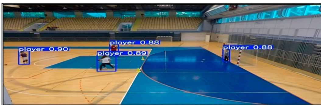
Figure 3. Example of player detections in a broadcast frame (YOLOv8 outputs).
