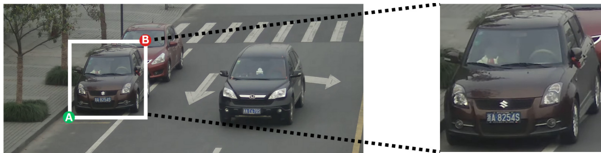
Figure 7. Algorithm 1 enables users to define a region of interest (ROI) by dragging the cursor from point A to point B (or vice versa).
