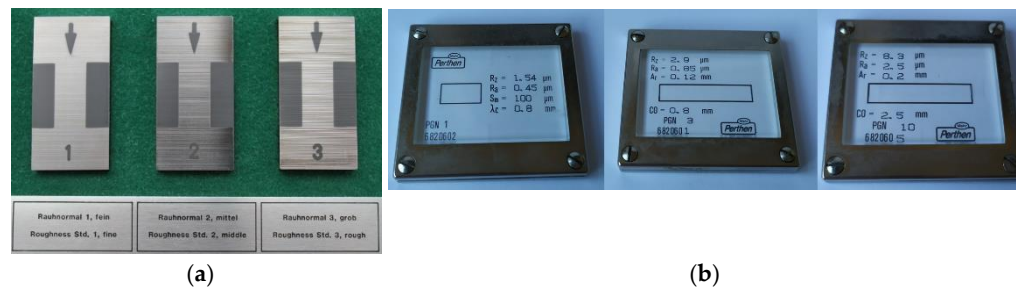
297 Figure 10. Step height standards used during calibration. (a) aperiodic, metallic standards (b) 298 periodical, glass standards.
