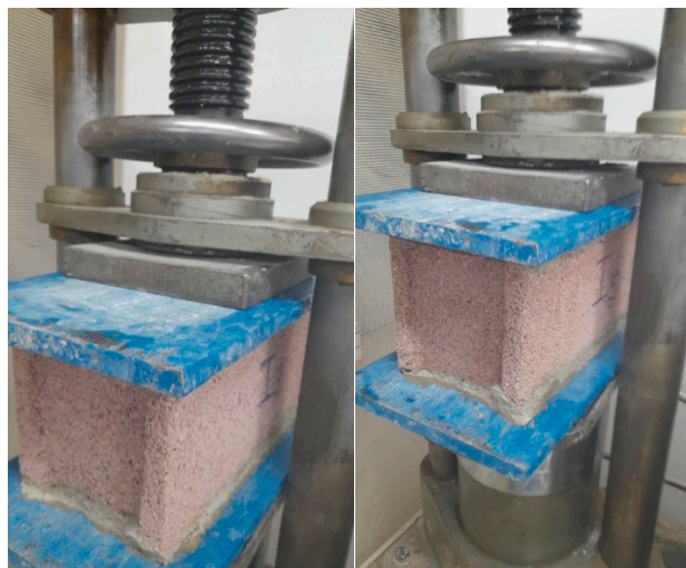
Figure 8. Determination of compressive strength of composite blocks according [22].
