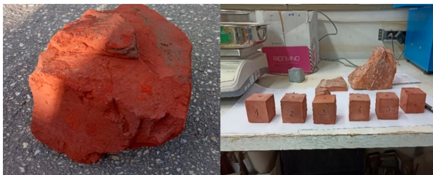
Figure 3. Irregularly shaped monolithic rock and cubic test samples 5x5x5 cm.
