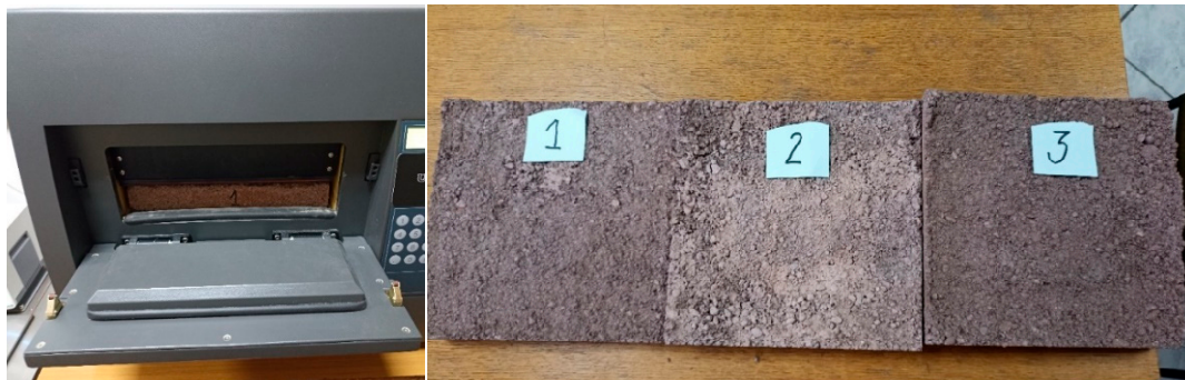
Figure 9: Instrument Heat Flow Meter and three testing samples.
