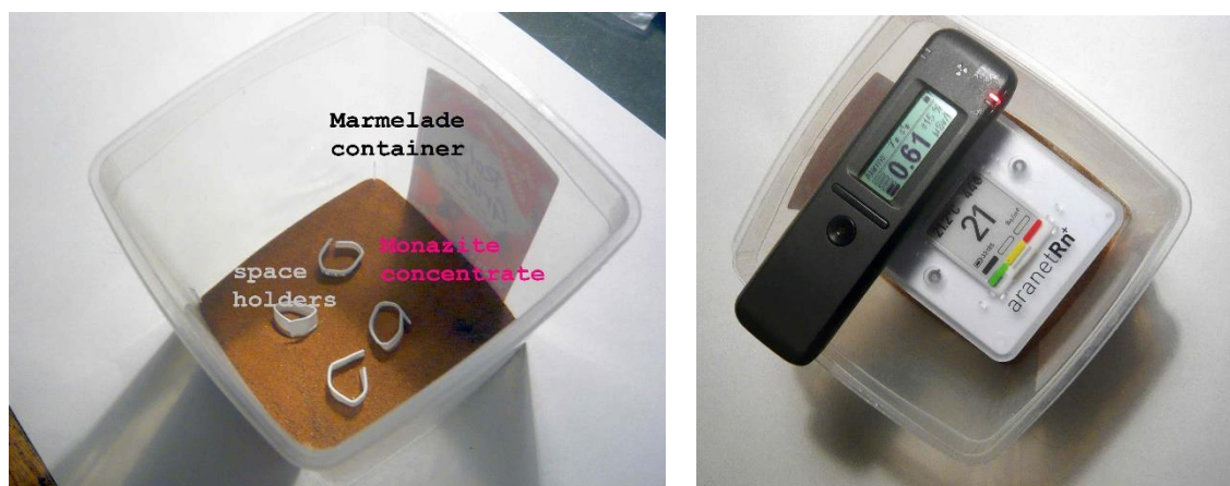
Figure 3. Exposure to thoron. Left – the plastic container with monazite concentrate; right – the Aranet monitor inserted. On top a Radiacode dose rate monitor ( \mu\text{Sv/h} ). During exposure the container was covered.
