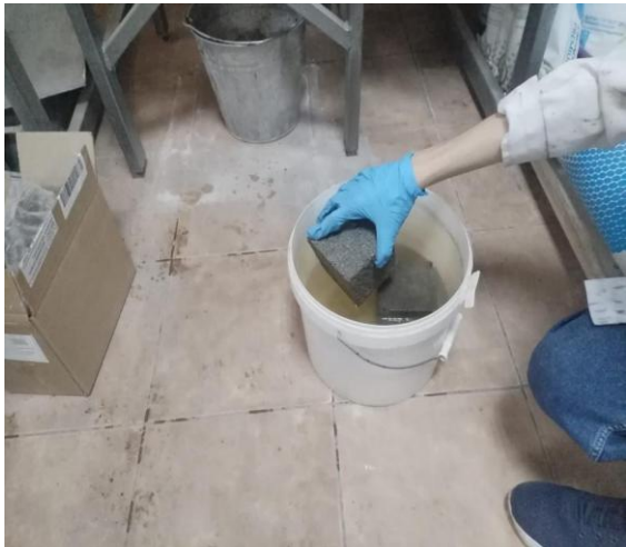
Figure 4. – Determination of water absorption of foam concrete samples.
