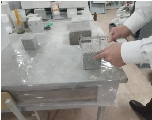
Figure 2. – Determination of the density of foam concrete samples.
