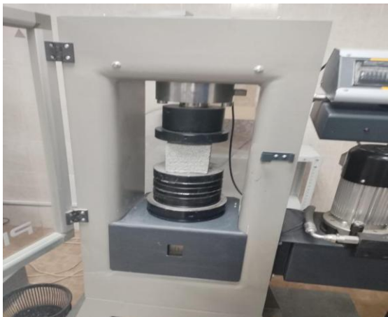
Figure 3. - Determination of strength of foam concrete specimens.
