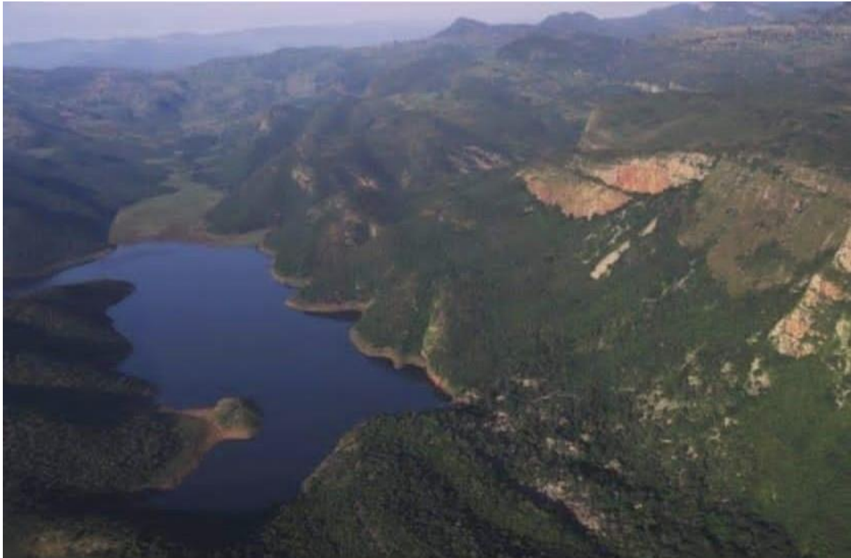
Figure 8: Lake Fundudzi a landslide dam on the Mutale River. Please note the tail end of the lake, which shows considerable sedimentation, which is due to ecological degradation of its catchment, as a result of commercial plantations and human settlement (Map, courtesy of Munyadziwa Magoma).
