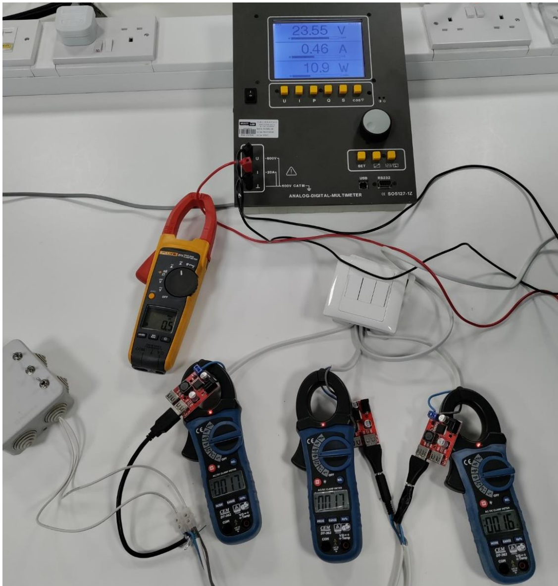
Figure 9. Experimental set-up of load sharing between parallel Buck cells
