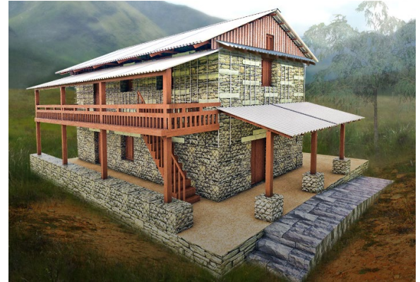
Figure 7 (b): 3D of Proposed Gabions Self-Built House
