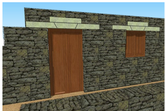
Figure 8 (b): Gabion Openings
